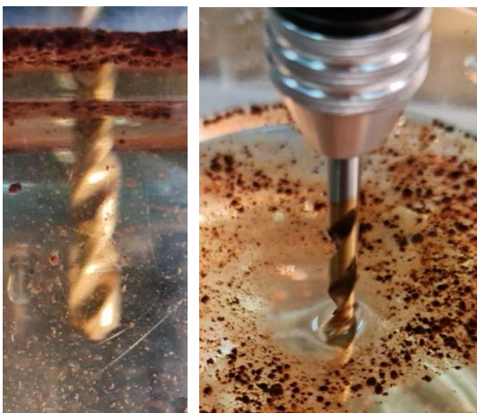
Figure 9. Rotation of the drill bit and highlighting the introduction of a quantity of water without coffee granules by removing the coffee granules as a result of the rotation of the drill bit (diameter of the drill bit: 3.2 mm; speed of the drill bit: 30 rev/min)
