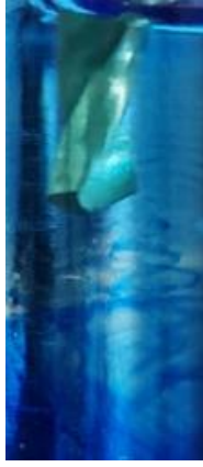
Figure 8. Rapid dissipation of the aqueous solution of blue ink dropped with the pipette in the area near the driven drill in rotational motion
