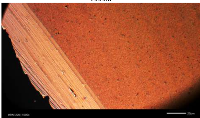
Figure 7. Deposition with ECWCL, optical microscopy, 1000x.
