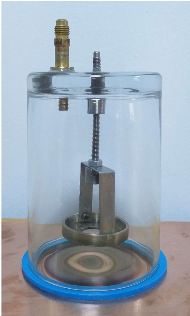
Figure 1. Sputtering with the experimental device.
