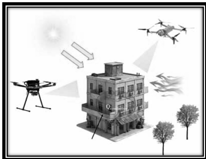
Figure 7. Detection and assessment of building defects and related equipment through 3D thermography using drones [22]
