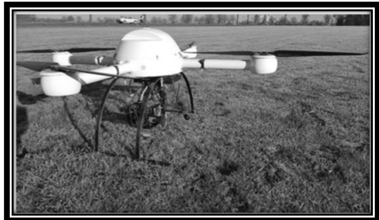
Figure 3. M4-1000 UAV (Microdrones) fitted with thermal and RGB imaging sensors [13]
