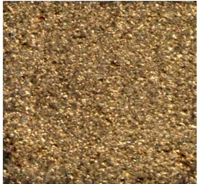
Figure 16. General view of the surface layer obtained by the method of metallic powder deposition using pulsed discharges with contact break (Cathode – Steel 45; Anode – BrOṬS-5-5-5; Metallic powder – BrA-7; Magnification \times 20 .)
