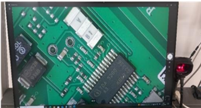
Figure 16 Checking the solder under a microscope
