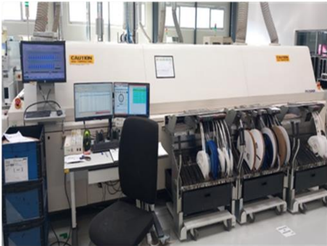
Figure 9 Electric reflow soldering oven TSM N70-i123MH
