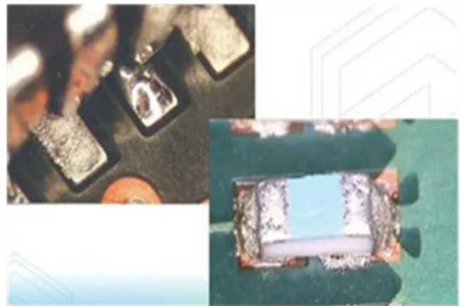
Figure 23 Cold solder joints
