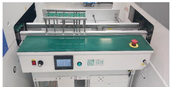
Figure 8 Transfer conveyor belt
