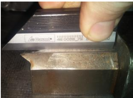
Figure 6. Missing material (cutter).
