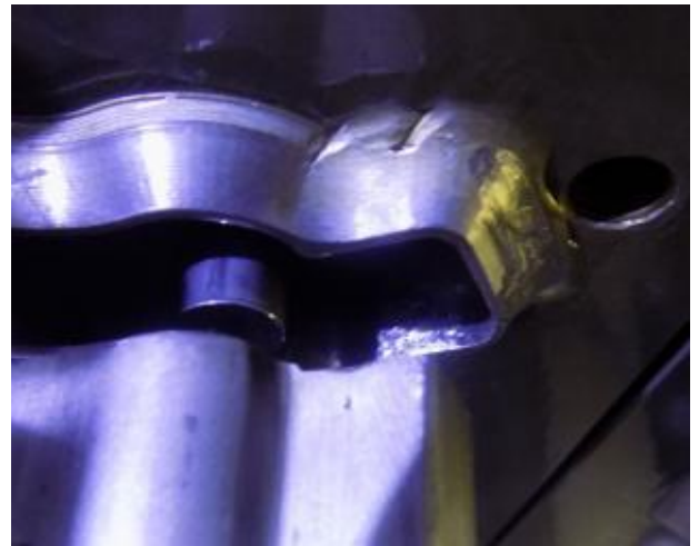
Figure 9. Worn out (upper cutter).
