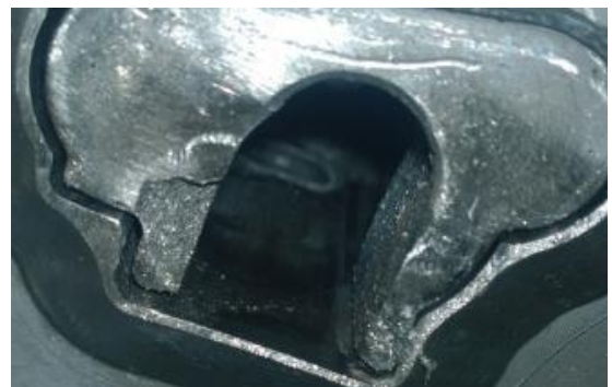
Figure 10. Worn out (cutter).
