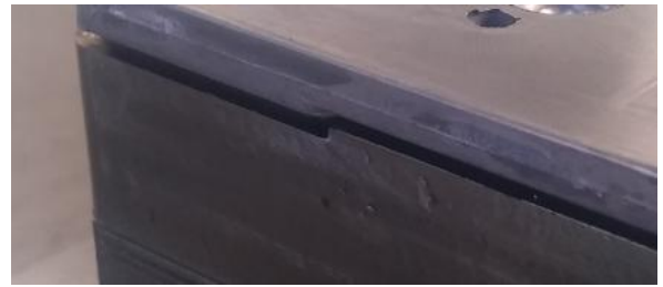
Figure 12. Distance between the support and part, caused by temperature.
