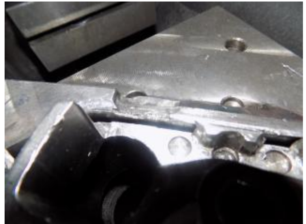
Figure 8. Worn out (lower cutter).
